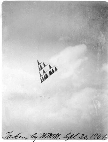
Fig. 6: Generation 2 kite designed by Alexander Graham Bell in flight [12].
