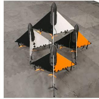
Fig. 10: An assembly of four *TetraDrone* single-modules.
