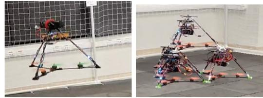
Fig. 7: Modified tetrahedral design of the *Tetracopter*. Left: Generation 1 Module in-flight. Right: Generation 2 vehicle in-flight.
