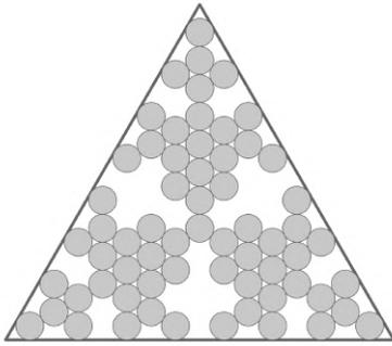
Fig. 5: Horizontal footprint of 3rd generation drone with 64 propellers.
