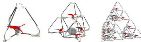
Fig. 4: Sierpiński tetrahedron-shaped modular drone. Left: single module. Middle: First-generation drone. Right, second-generation drone.
