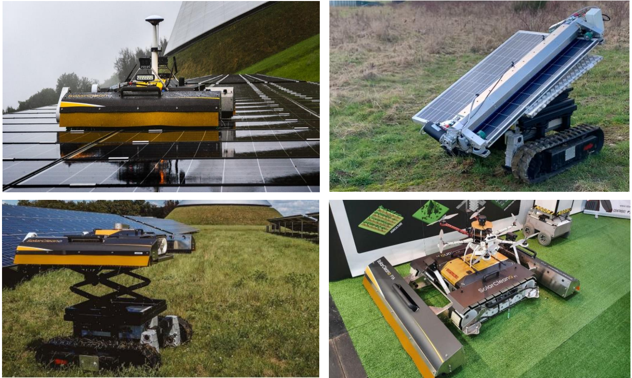
Fig. 1. System architecture of the MRS for solar panel I&M. top left) F1A; top right) R1A; bottom left) T1A; bottom right) U1A.
